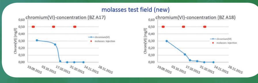
Fig. 14: Very good reduction results with molassis in the new larger test field
