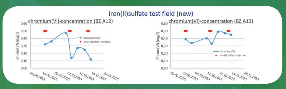
Fig. 15:: Insufficient chemical reduction results downstream
