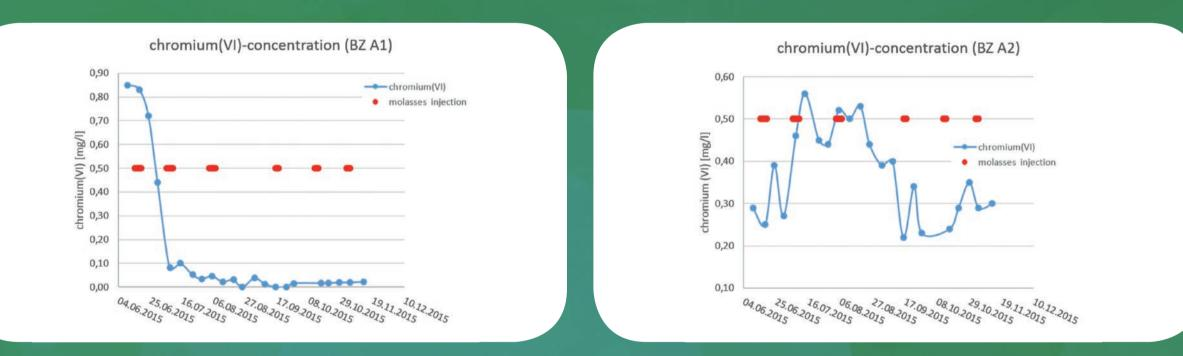
Fig. 10: Quick chromium reduction and immobilization with molassis in the field test area 1
