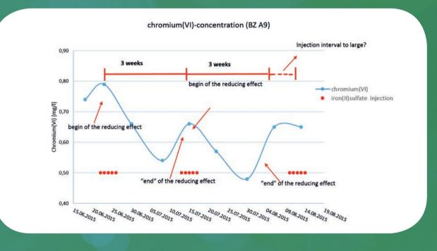
Fig. 11: Insufficient chromium reduction / immobilization with iron(II)sulfate in the field test area 2
