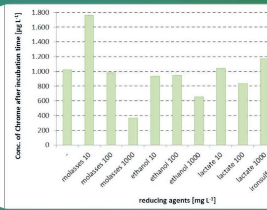
Fig. 5: Different chemical and biological reducing agents tested in 3 different concentrations using 48-h-shaked batch tests
